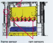
The sensor type and its position are determined by the respective monitoring task.
